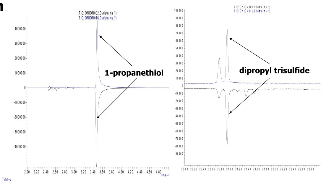
The figure on the left displays the retention time region for the primary odorant compound  $\rightarrow$  1-propanethiol. The figure on the right displays the retention time region for another 1<sup>st</sup> tier odorant compound  $\rightarrow$  dipropyl trisulfide.
