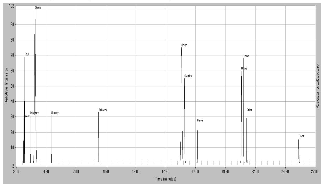
Olfactory analysis was performed simultaneously during the GC/MS analysis to detect the compounds that contribute to the aroma of the red onion. An aromagram is a graphical representation of this olfactory analysis. Each peak indicates a presence of an aroma compound that was sensed at the Sniff Port (olfactory detector) by the scientist at the
